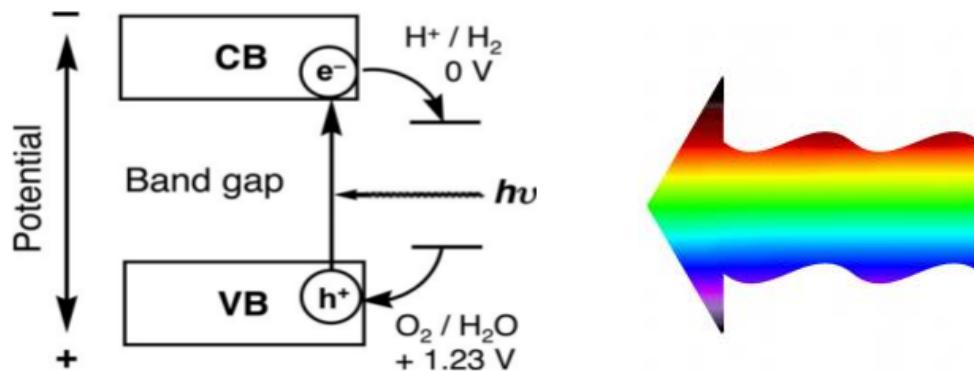
Principle of water splitting using semiconductor photocatalysts.
